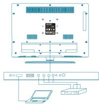
1. Connect the TV RF source to the RF IN port. TVRF signal including: Receiving antenna /satellite TV/CATV net. You can use  $75\Omega$  coaxial cable to connect the outdoor antenna.
